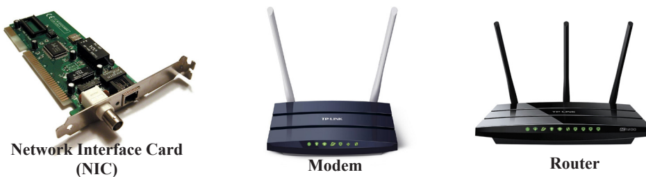
Figure 1.9 - Wired/Wireless Communication Devices
